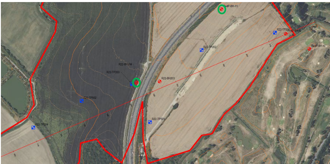
Plate 4: Plan of boreholes and transects. Thanet Formation was record directly below the topsoil in the boreholes circled in green.
