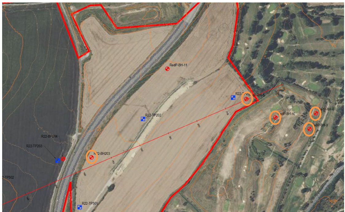
Plate 6: Plan of boreholes and transects. Alluvium/ Tidal Flat Deposits were identified in those boreholes circled in orange.
